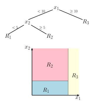
To use a regression tree, there are 2M quantities to be determined: the regions  $R_1, \dots, R_M$  and the predicted values  $c_1, \dots, c_M$ . When  $R_1, \dots, R_M$  are given,  $c_1, \dots, c_M$  can be simply estimated by the average within each region, i.e.,
