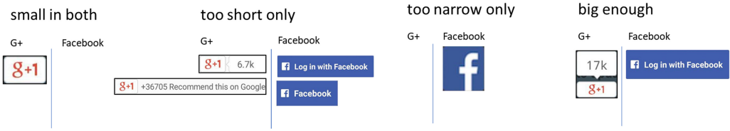
Fig. 19. Sample Google+ (g+1) and Facebook Login elements that had the size-based errors of being too small in both , too short only , too narrow only , or big enough , based on Android Accessibility Guidelines [9]. The comparison highlights how design choices made by third-party providers can impact many apps.
