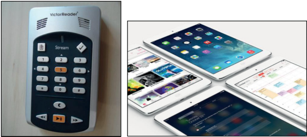
Fig. 1. Left: The VictorReader Stream (VRS), a digital music player for the visually impaired that also plays audio books. Right: A mainstream counterpart, the Apple iPad Air, allows users to play music, read books, and interact with many other kinds of digital content.
