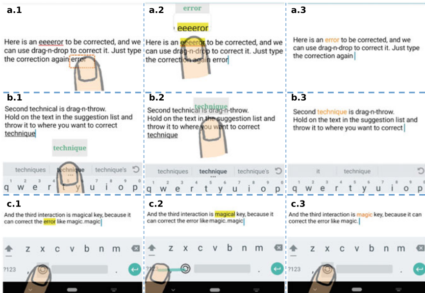
Fig. 3 The three interaction techniques. Drag-n-Drop : a.1 Type a word and then touch it to initiate correction; a.2 Drag the correction to the error position. Touched words are highlighted and magnified, and the correction shows above the magnifier; a.3 Drop the correction on the error to finish. Drag-n-Throw : b.1 Dwell on a word from the suggestion list to initiate correction. The word will display above the finger; b.2 Flick the finger toward the area of the error: here, the flick ended on “the,” not the error text “technical”; b.3 The algorithm determines the error successfully, and confirming animation appears. Magic Key : c.1 Tap the magic key (the circular button) to trigger correction. Here, “error” is shown as the nearest potential error. c.2 Drag left from atop the magic key to highlight the next possible error in that direction. Now, “magical” is highlighted. c.3 Tap the magic key again to commit the correction “magic”
