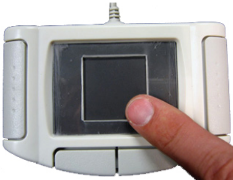
----- Figure 4: EdgeWrite on a Synaptics TouchPad with a plastic template with a square hole. -----
