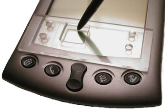
----- Figure 1: The Square Template in EdgeWrite for Stylus Input on a Palm PDA -----
