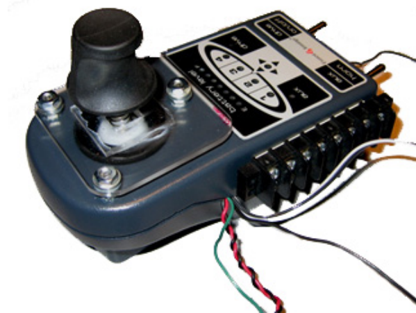
Figure 6: The Everest & Jennings 1706-5020 power wheelchair joystick we modified for EdgeWrite text entry. Note the plastic template around the stick, which provides a square boundary.
