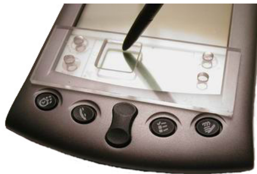
Figure 3: A Palm PDA with an EdgeWrite template over the text input area. A user makes all letters, numbers, and punctuation inside the square hole by moving the stylus along the edges and across the diagonals of the square. Small holes in the template provide access to the four soft buttons on the Palm.
