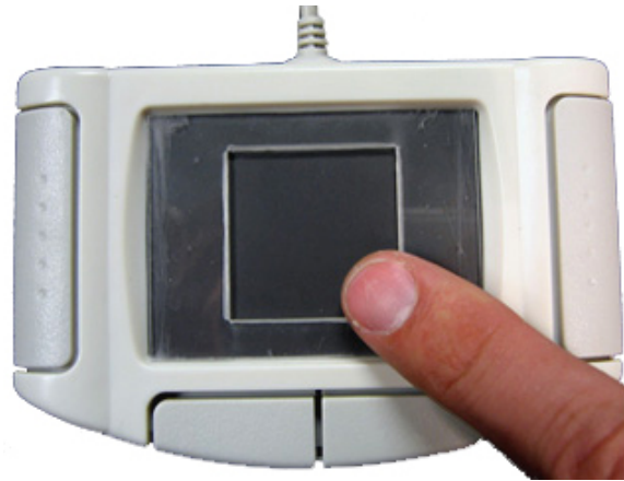
Figure 7: The Synaptics touchpad we used with a plastic template to create a square area for EdgeWrite text entry.
