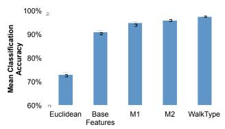
**Figure 4.** Classification accuracy with different models. M1 is the Displacement and Acceleration Model and M2 is the Walking Pattern Model. The difference in performance of Base Features and WalkType illustrates the benefit of the accelerometer data. Error bars show standard error.
