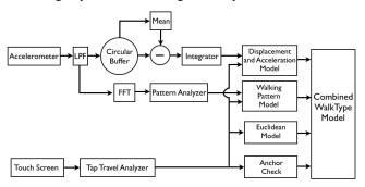
**Figure 7.** Block diagram of major components of WalkType's Model Building phase.
