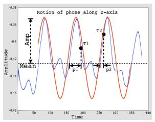
**Figure 5.** Motion of the phone along *z*-axis when the user is walking. T1 and T2 are two instances of taps; p1 and p2 are the elapsed times since the signal crossed the mean. The waveform in red is part of the dominant frequency wave.
