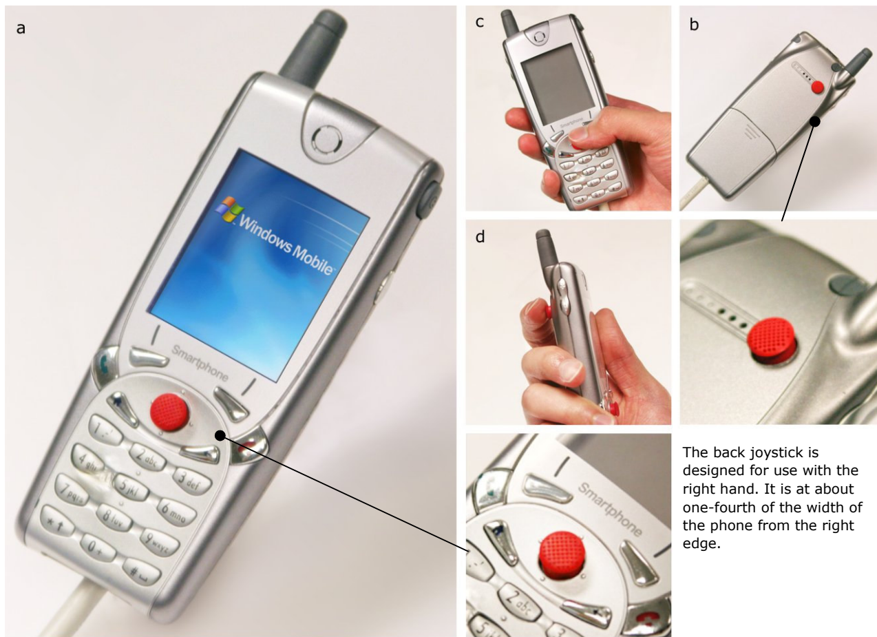
Figure 1a. front view. Almost all of the original phone components are preserved. The LCD screen is fully functional. The two joysticks communicate with a computer through a PS/2 connection using the cable at the bottom of the phone. b. back view. c. the thumb operating the front joystick. d. the index finger operating the back joystick.
