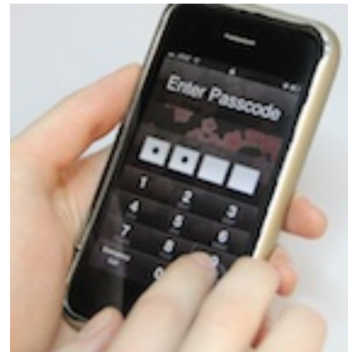
Figure 1: When entering passwords with an iPhone and VoiceOver, a user's input is spoken as she touches the screen, posing a severe security risk.
