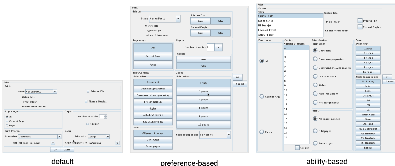
Figure 3: Three user interfaces for a print dialog box: a default reproduced from Microsoft Word 2003 and two automatically generated for a user with impaired dexterity: one based on his subjective preferences as elicited by ARNAULD, and one based on his actual motor abilities as modeled by SUPPLE++.
