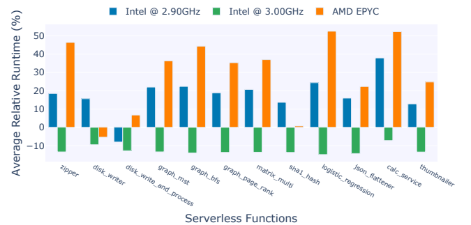
Figure 9: Workload performance normalized to the performance of the 2.5 GHz Processor on AWS Lambda.
