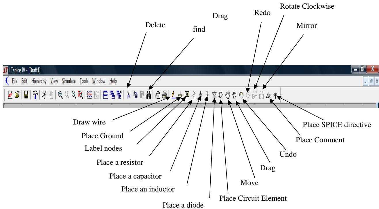
To place circuit elements beyond those shown on the main menu, we click the button **Place Circuit Element** and we select the desired element from the list of elements that appears in a window that looks like the figure shown below.
