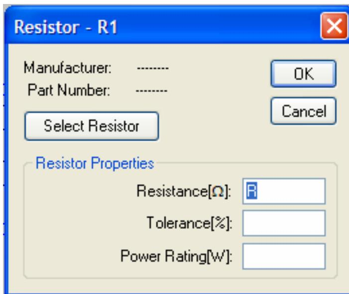
To change the value of the resistor enter the value in ohms in the entry for resistance or press the **Select Resistor** button and choose the value from the list that appears.
