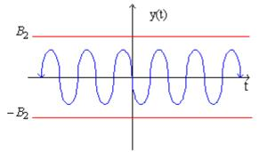
Ex. Resistor is stable V=iR,  $|i(t)| \leq B_1 \rightarrow |v(t)| \leq RB_1$
