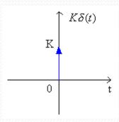
The pulse height gets higher and higher and its width goes to zero, but its area is still 1! So define  $\delta(t)$  as unit impulse:
