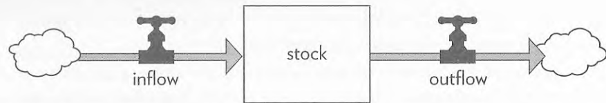
Figure 1. How to read stock-and-flow diagrams. In this book, stocks are shown as boxes, and flows as arrow-headed “pipes” leading into or out of the stocks. The small T on each flow signifies a “faucet;” it can be turned higher or lower, on or off. The “clouds” stand for wherever the flows come from and go to—the sources and sinks that are being ignored for the purposes of the present discussion.
