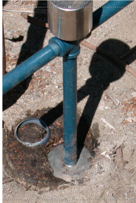
Soil sample collection (a) water infiltration ring, (b) bulk density core and intact core used for water holding capacity and microbial activity, and (c) collecting cores for soil chemical analysis including total C and N and available nutrients
