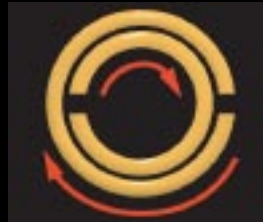
Circular currents flow in split-ring resonators (SRRs).
