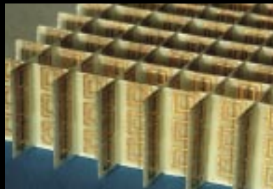
A metamaterial is made by creating an array of wires and SRRs that are smaller than the wavelength of the electromagnetic waves to be used with the material.
