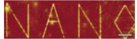
35-nanometer layer of silver in place ( right ). Scale bar is 2,000 nanometers long. With the superlens, the resolution is finer than the 365-nanometer wavelength of the light used.
