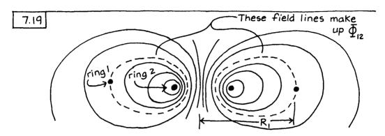
The point is that the flux which links ring 2 is determined by the lines of force, in the field of ring 1, which return outside ring 2. That is why  $\Phi_{12}$  decreases as  $R_1$  increases, holding  $R_2$  and  $\Gamma_2$  constant.
