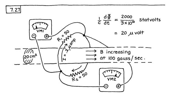
The loop that includes R, and VMI encloses no changing flux. The potential drop across R, is  $10\mu\nu$ , with the more positive end connected to  $\Theta$  terminal on VMI. Hence VMI will read  $-10\mu\nu$ olt. The loop that involves R, and VM2 encloses changing flux. The line integral of E around that loop includes  $+20\mu\nu$  in addition to the -10 across R, VM2 will read  $+10\mu\nu$ olt.
