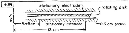
With the disk at 10 kv, the electric field strength in the space above and in the space below the disk is:
