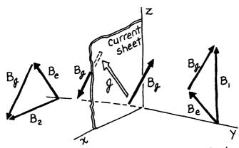
The statement on p. 234 that  $(B_1^2 - B_2^2)/8\pi$  is the force per cm² would imply that the force is zero in this case where  $B_1^2 = B_2^2$  although  $B_1 \neq B_2$ . Indeed that is true, for what we have here is a superposition of the field of some external source  $B_e$ , the same on both sides of the sheet, and  $B_g$ , the field of a current f flowing in the sheet. If f is parallel to f there can be no force on the sheet.
