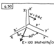
In frame F,  $E_{x} = 100 \cos 30^{\circ} = 86.6$ ; Ey = 100 sin 30° = 50; E, = 0; B = 0 Eq. 58 is the transformation for motion of F' in the x-direction.
