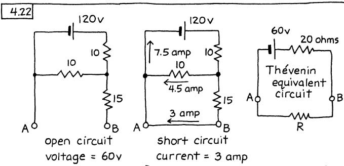
For max. power in R: R= 20 ohms; P = 45 watts
