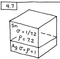
The ratio of conductivities, 7.2/1 and the ratio of layer thicknesses, 1/2, is all that matters. Let's take  $\sigma_{Ag} = f_{Ag} = 1$  and consider the cube that is 1/3 silver, 2/3 tin. For vertical currents the layers are in series and resistances add:
