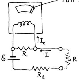
The current I in the external circuit will be 0.1 amp, in order of magnitude, if adding 15 ohms cuts it in half. This is very much larger than 50 µ amp. This tells us the resistance R, must be  $\ll R_c$ , so that nearly all of the
