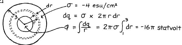
Electron's final K.E. =  $e \phi = 4.8 \times 10^{-10} \times 16\pi = 2.41 \times 10^{-8}$  erg Electron rest energy mc<sup>2</sup> =  $81 \times 10^{-8}$  erg. Since K.E./mc<sup>2</sup>  $\approx 0.03$  a non-relativistic calculation should be good enough:
