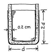
1 liter =  $10^3$  cm<sup>3</sup> =  $2d \times \frac{\pi}{4}d^2$ , or d = 8.6 cm area of capacitor =  $\pi d \times 2d + \frac{\pi}{4}d^2 = \frac{9}{4}\pi d^2$  = 522 cm<sup>2</sup>
