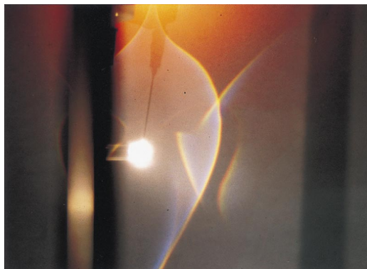
Fig. 6. Rainbow caustics of a single water droplet, illuminated by white light from an arc lamp.
