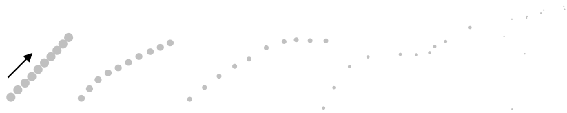
Figure 3: Trajectories are changed when one tries to measure them too accurately: A series of position measurements, with a precision given by the gray circles, is carried out in constant time intervals. When the spatial resolution is increased (from left to right), the random deflections in momentum at each step are also enlarged, which finally leads to something like a random walk.
