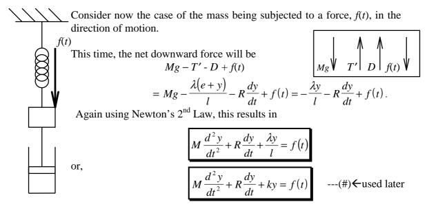
Note how the only difference here is that *the input to the system*, f(t), the forcing term, appears on the right hand side of the differential equation rather than the zero when the system was unforced (i.e. zero input).
