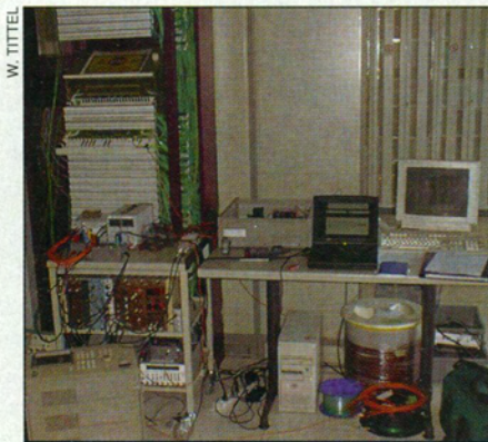
Photons phone home. A photon source (on table), plugged into the Geneva telephone exchange (far left), sends pairs of correlated photons to two nearby villages (map).
