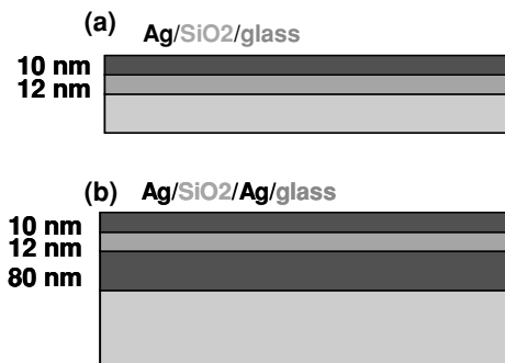
Figure 14.6. Vertical layer structure for ASF substrates: (a) two-layer structure, (b) sandwich structure with an additional thick metal sublayer.
