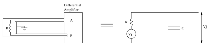
FIG. 1: Equivalent circuit of the thermal emf across a conductor of resistance R connected to a measuring device with cables having a capacitance C
