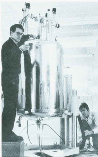
Superconducting magnet for a Bruker 600-MHz spectrometer. (G. Clore, left, and A. Bax of NIH)
