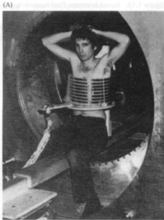
Figure 1.14 The first MR image of the human body. Raymond Damadian and colleagues constructed an early large-bore MRI scanner, which was called "Indomitable." Larry Minkoff, a postdoctoral fellow in the laboratory, was the first subject from whom data were recorded (A). The resulting image of his chest (B), while primitive by modern standards, shows the heart, lungs, and surrounding musculature. (A from FONAR corporation; B from Damadian et al., 1977)
