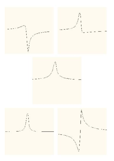
One can think of the *real*( $\omega$ ) and *imaginary*( $\omega$ ) as the spectra seen by the two detectors - they are necessary 90 dephased. The phase is given by the position of the global magnetization **M** at the beginning of the acquisition. The zero-order correction (**rp**) takes care of the dephasing between the transmitter and the reciever.
