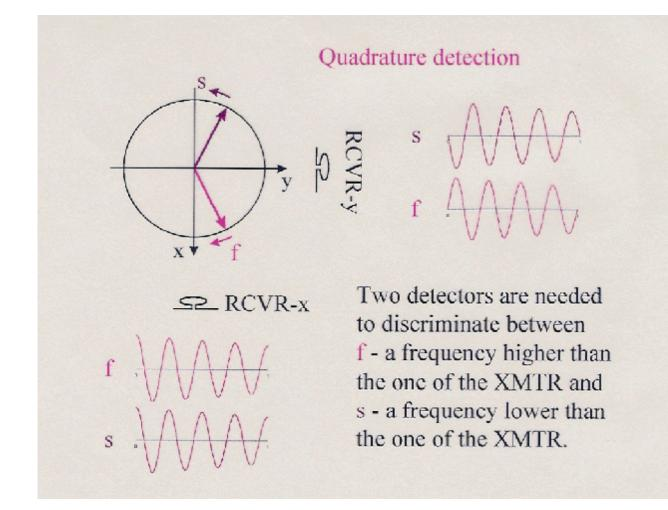
Physically a second detector, is realized by combining the signal with the transmitter frequency, shifted by 90.
