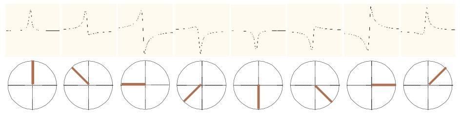
The first-order correction (Ip) takes care of the dephasing of the frequencies between the middle of the pulse and the beginning of the acquisition.
