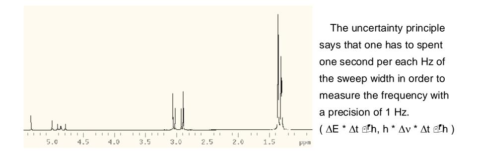
A 15 ppm sweep width at 300 MHz takes 4500 s per scan for a poor resolution of 1Hz !
