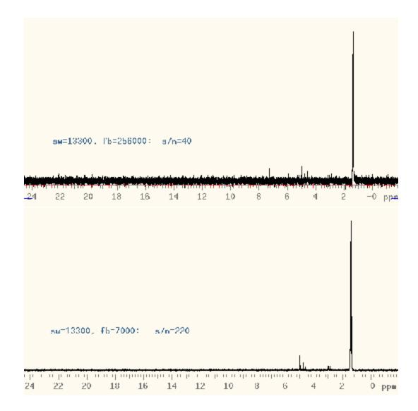
➤The spectral window is defined by sw and tof (the frequency of the pulse, which is the center of the spectral window).
