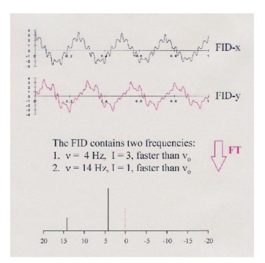
The Cooley-Tuckey algorithm transforms an FID of np=2<sup>n</sup> points into a spectrum of fn=2<sup>n</sup> points.
