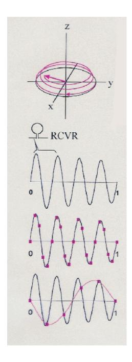
At 300 Mhz, 1/DW should be >600 MHz. Actually the ADC is 100 kHz.
