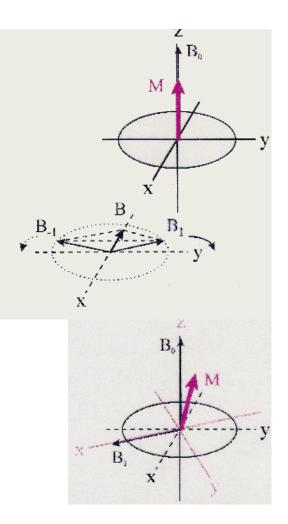
>In the laboratory frame, M rotates simultaneously about two axes,  $B_0$  and  $B_1$ .
