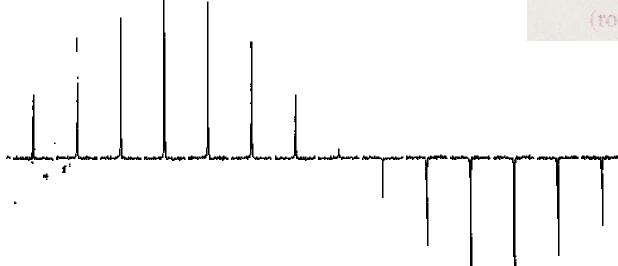
>For a real sample, with more than one signal, B<sub>1</sub> precesses with  $\omega_0 = \gamma$ B<sub>0</sub> while M precesses with  $\omega = \gamma$  B<sub>eff</sub>. Consequences:
