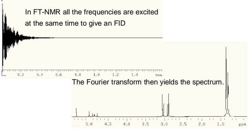
A 15 ppm sweep width at 300 MHz takes **1 s** per scan for a poor resolution of 1Hz !
