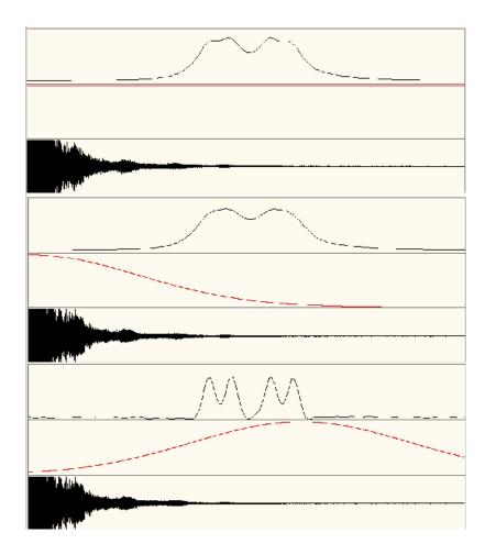
One can improve the resolution or the signal to noise ratio by multiplying the FID with a window function prior to Fourier transform. Like this one can increase the weight in the spectrum of the first part of the FID (good s/n) or of a later part (good resolution).
