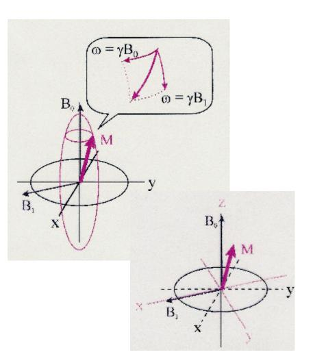
The intensity of the signal is proportional to the projection of M into the xy plane:  $M_y$ = M cos( $\gamma$  B<sub>1</sub>t).
