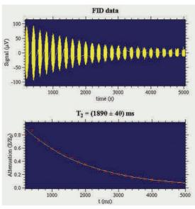
Typical results for a measurement of the  $T_2$  of a tap water sample using the CPMG sequence. These results were obtained in de-shimmed conditions.
