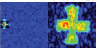
A 2D spin-echo image of a potato cut into the shape of a Maltese cross . On the left is the k-space data of echoes and on the right is the 2D Fourier transform of the data to show the MRI of the potato. Imaging time was 4 min.
