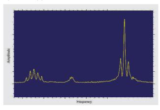
Heteronuclear *J*-couplings observed simultaneously between  $^{19}$ F and  $^{1}$ H in 1,4-difluorobenzene. The four-proton triplet is observed on the right at 2425 Hz and two atom  $^{19}$ F quintuplet at 2275 Hz on the left. (A 50 Hz noise harmonic is visible near the centre.)
