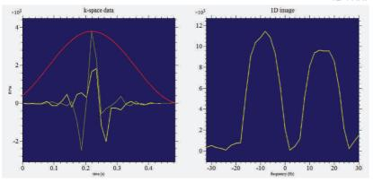
A 1D imaging sequence using a spin echo and a single gradient. On the left is the acquired echo and on the right is the Fourier transform of the echo showing the 1D projection image. The sample shown here is the two tube phantom supplied with the Terranova-MRI.
