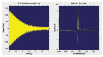
An FID of a water sample collected for 3 seconds to show the enhanced amplitude and linewidth obtained following shimming and tuning. (Note that the data has been processed in complex rather than magnitude mode - this enables the linewidth to be correctly determined).
