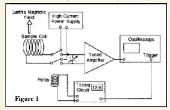
The high Q sample coil surrounds a 125 ml plastic bottle containing a liquid rich in either hydrogen or fluorine nuclei. The sample is placed in a uniform part of the earth's magnetic field with the coil's axis aligned perpendicular to this field. The sample coil is connected first to a current
