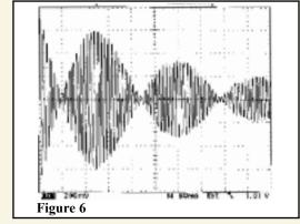
6. Precession Frequency Gives Local Magnetic Field Using the gyromagnetic ratio  $\gamma$  of either the proton
