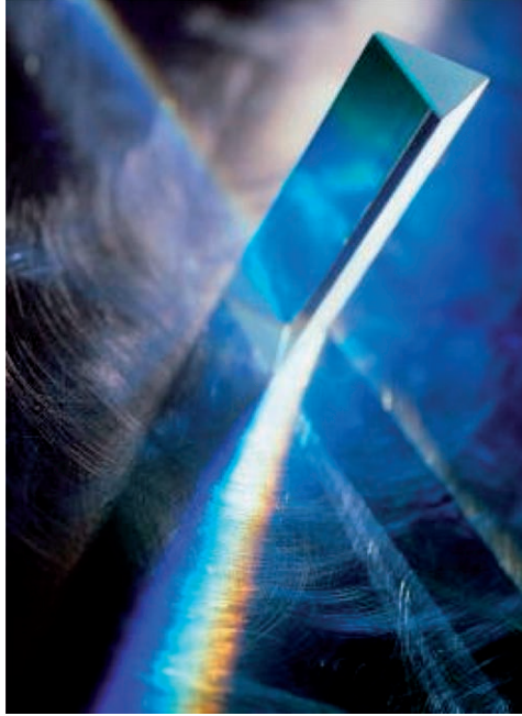
Figure 5.1 A prism performs spectral decomposition of white light in bands with different wavelengths that are perceived by us as different colors.
