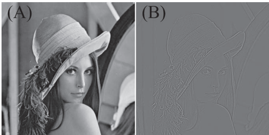
Figure 13.4 An example of a filter application in the spatial domain using a picture of Lena (A) as input for a two-dimensional Butterworth high-pass filter. Although this spatial filter is not optimized for this application, by using the principle of high-pass filtering we can detect transitions (edges) in the spatial domain as shown in (B).
