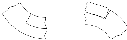
Figure 9.34. Bending of the inserts in the first gap element for positive and negative beam curvature.
