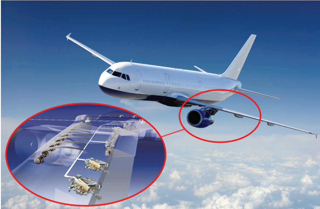
Aircraft actuation systems require embedded condition monitoring and load sensing devices. Courtesy of Moog Inc. and airline photo from iStock.
