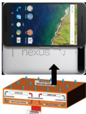
*Ultra-thin heat pipe devices may enable higher performance mobile electronic devices that are cool to the touch.*
