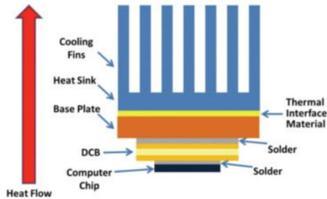
*Schematic of electrical, thermal, and mechanical system needed for a computer chip to function. Solder and thermal greases play critical roles in heat flow from the chip to the outside air. Transient liquid phase sintering systems can replace both solder and thermal interface materials, increasing bond performance at higher temperatures needed for automotive and power electronics applications.*
