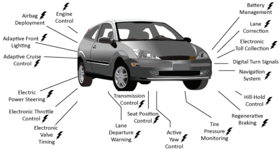
*Smart cars contain multiple embedded electronic control units. The concern is that multiple ECUs that have different non-transferable functions result in highly failure-susceptible systems.*
