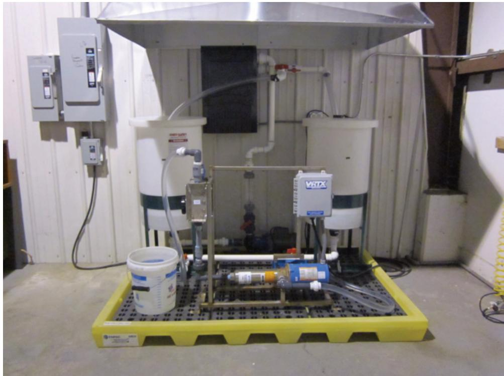
*The laboratory set-up of individual components used in the Advanced Water Treatment skid. The hydrodynamic cavitation unit is at the forefront, the UV-ozone generator is mounted on the wall, and two storage containers for testing the real produced water. The electrochemical cell along with hydrodynamic cavitation unit and UV-ozone generator form the Advanced Water Treatment skid.*
