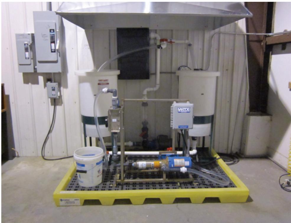
*The laboratory set-up of individual components used in the Advanced Water Treatment skid. The hydrodynamic cavitation unit is at the forefront, the UV-ozone generator is mounted on the wall, and two storage containers for testing the real produced water. The electrochemical cell along with hydrodynamic cavitation unit and UV-ozone generator form the Advanced Water Treatment skid.*
