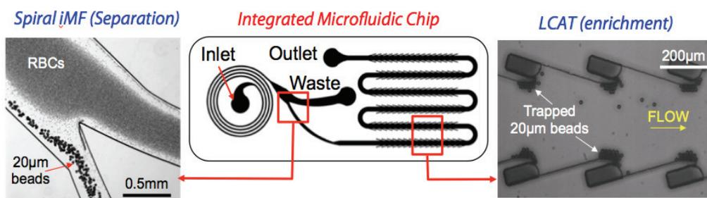
*20µm-diameter beads separate from whole blood due to inertial forces (RBC = red blood cells). 20µm-diameter beads get trapped in the microvortices of LCAT as they pass through the main flow channel.*
