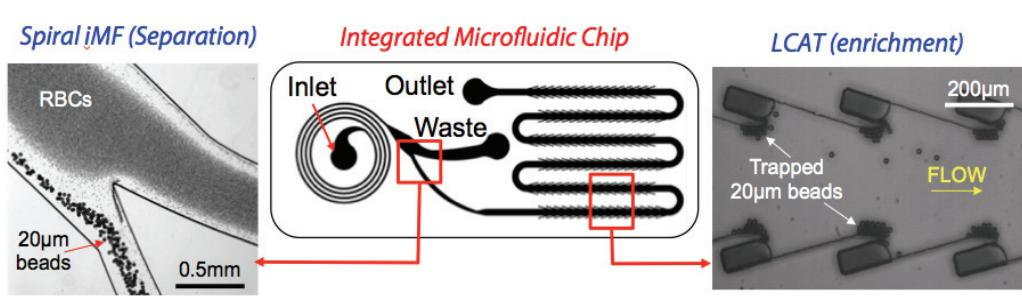
20 $\mu$ m-diameter beads separate from whole blood due to inertial forces (RBC = red blood cells). 20 $\mu$ m-diameter beads get trapped in the microvortices of LCAT as they pass through the main flow channel.
