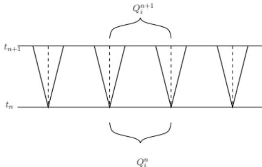
Data at time  $t_n$ :  $\tilde{q}^n(x, t_n) = Q_i^n$  for  $x_{i-1/2} < x < x_{i+1/2}$
