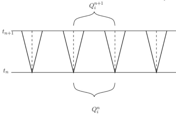
$$\tilde{q}^n(x_{i-1/2}, t) \equiv q^\psi(Q_{i-1}, Q_i) \text{ for } t > t_n.$$
