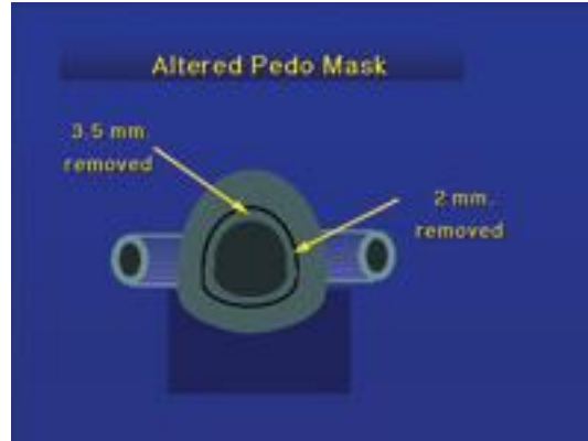
Figure 13. By altering the shape and size of the nose hole, a pediatric mask can be used by adults.
