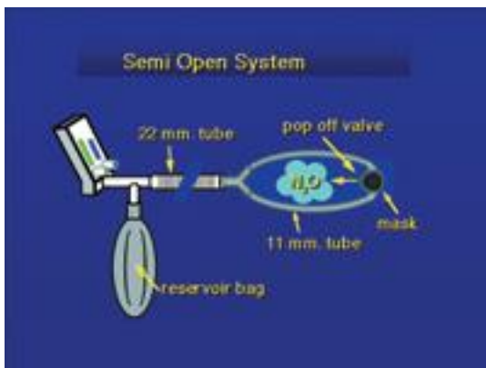
Figure 6. The semi-open system allowed gas to escape from a pop-off valve on the mask and into the breathing space of the dentist and dental assistant. This led to nitrous oxide levels as high as 5,000 ppm.
