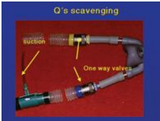
Figure 12. By adding a hose, two one-way valves, and suction, a semi open system can be converted to a scavenging system.
