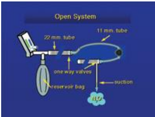
Figure 11. In the open system, gas is drawn from the bag and exhaled through a second hose, or into a space around the mask. Suction then removes the waste gas.
