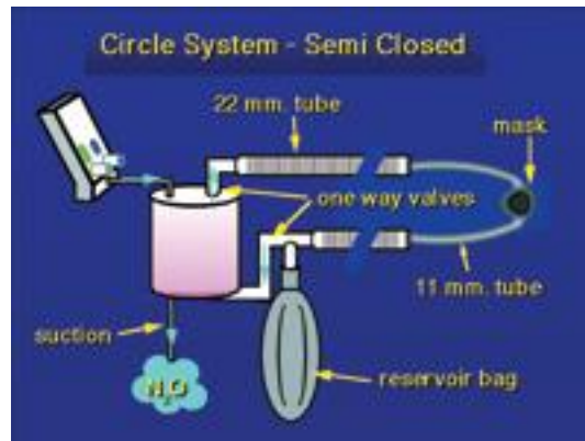
Figure 8. Semi-closed or circle system with a CO 2 absorbing canister. The gas is reused, removing CO 2 each time the gas passes through the soda lime granules in the absorber canister. This system requires a nitrous oxide machine that can deliver low flow volumes.
