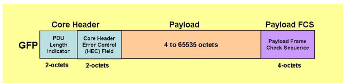
Figure 6 ITU-T G.7041/Y.1303 GFP Framing where interfaces for G.709 is specified for OTN
