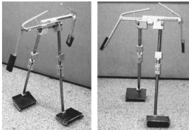
Fig. 3. Our two-legged, kneed, passive-dynamic walking robot. The counter-swinging arms are attached rigidly to their opposing legs. Note that the right arm swings forward and out as the left leg swings forward.
