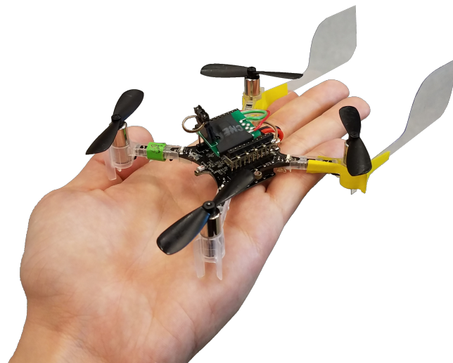
Fig. 1. The Smellicopter is a modified commercial Crazyflie drone with custom electroantennogram circuit and vanes for passive upwind orientation.
