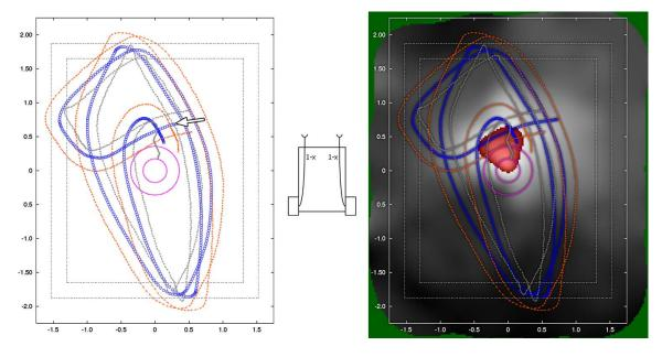
Fig. 5. Example of the path of a "permanent love" Braitenberg vehicle (uncrosssed (1-x)-connections) with the gas source in the middle of the testbed area.
