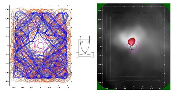
Fig. 8. Left side: path of a Braitenberg-Vehicle with crosssed (1-x)-connections ("exploring love") during a complete experiment, lasting 3 hours and including 5 separate trials. Right side: Concentration gridmap determined from the readings collected during the same experiment. The locations where the robot entered the clearance area around the gas source are indicated by small circles.
