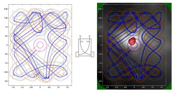
Fig. 7. Example of the path of a Braitenberg-Vehicle with crosssed (1-x)-connections ("exploring love") with the gas source in the middle of the testbed area.
