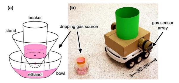
**Fig. 1.** Koala robot with the Örebro Mark III mobile nose and the dripping gas source used in the experiments. The gas source is schematically shown on the left side (a), and the robot is depicted in front of the gas source on the right side (b).
