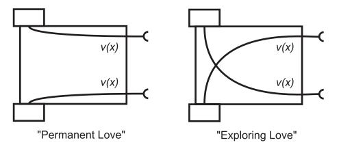
Fig. 3. Schematic view of Braitenberg vehicles with a direct inhibitory sensor motor coupling. Left: uncrossed connections ("permanent love"). Right: crossed connections ("exploring love").
