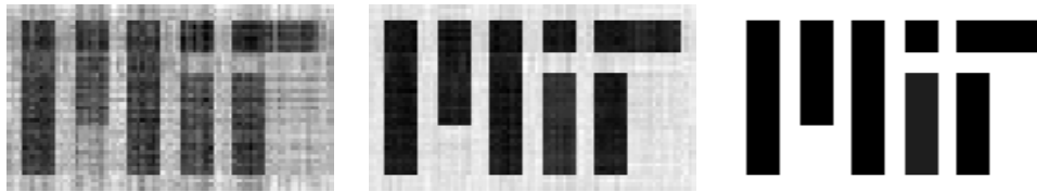
Fig. 3. Example recovered images using the Gaussian ensemble. (left) 700 measurements. (middle) 1100 measurements (right) 1250 measurements. The total number of pixels is 46 \times 81 = 3726 . Note that the error is plotted on a logarithmic scale.
