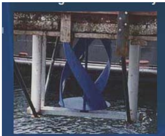
Figure 38: Vertical Axis Gorlov Helical Turbine 66
