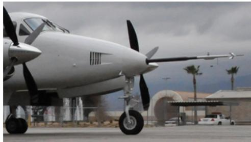
Fig. 6: Typical nose boom system setup.<sup>1</sup>
