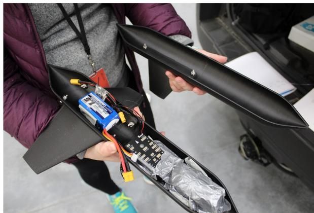
Fig. 30: The open model showing the internal configuration of the Pixhawk data acquisition system and additional payload.
