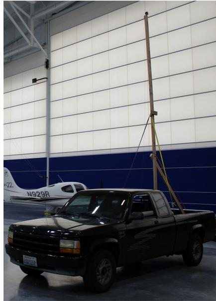
Fig. 29: Stability ground test model mounting system in place in the back of a pickup truck.
