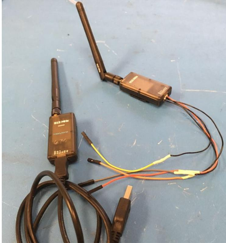
Fig. 16: Pair of 915MHz telemetry radios in kit.
