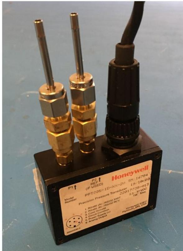
Fig. 14: Honeywell Precision Pressure Transducer.
