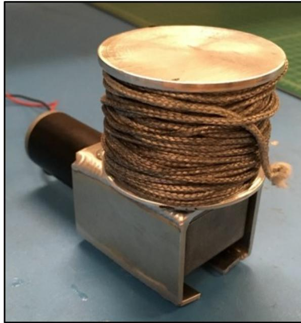
Fig. 22: Final winch as assembled.
