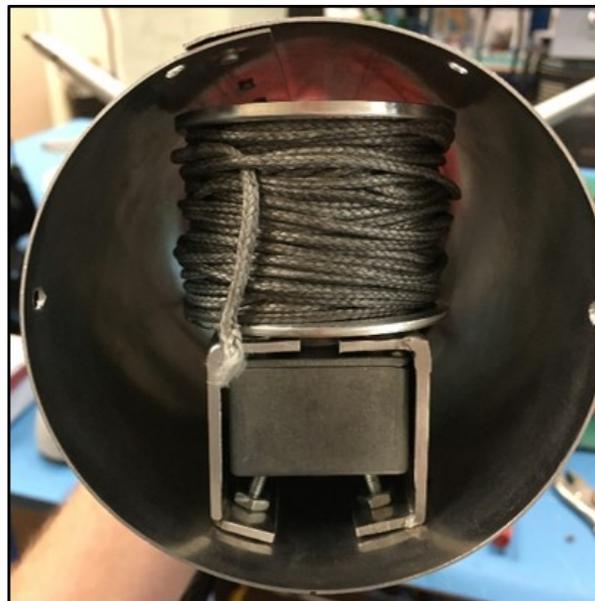
Fig. 23: Winch mounted inside fuselage.
