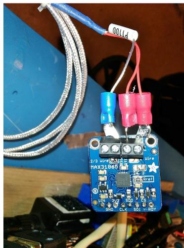
Fig. 15: MAX31865 amplifier board connected to PT100 RTD.
