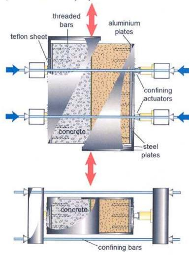
Two aluminium plates, cast together with the concrete blocks, are used to transfer the load from the steel frame to the specimen.
