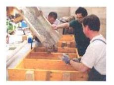
Place aluminium plate with threaded bars (for load transfer from steel frame to concrete)
