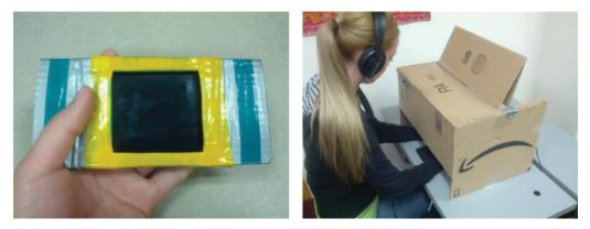
Fig. 1. Study 1 setup. (Left) Since the Samsung Galaxy Nexus screen has no tactile edge, we used a physical overlay to demarcate the active screen area. (Right) To impose eyes-free use, participants placed their hands inside of a box during tasks.
